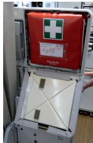
PNR 6240-87S • First Aid Kit stowed in A320 CAS headrest and hatrack lifeline spacer
